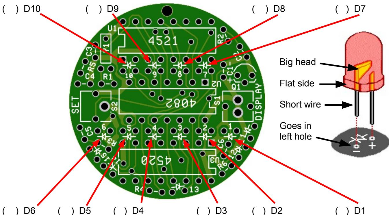
Install the ICs next. The ICs come with their pins bent slightly outward. To fix this, stand the IC on its side on the table, and tip it slightly inward so the rows of pins are parallel and will fit into the holes on the board.
