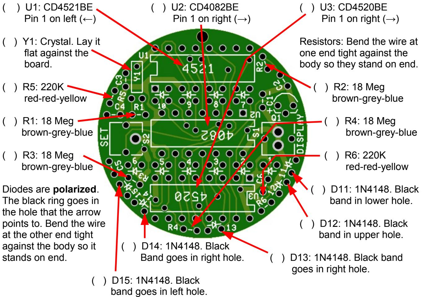
Install the capacitors next. Don't mix them up! There are tiny markings on them, but you may need a magnifying glass to read them. C1 is blue and **polarized**; it has a tiny "+" sign. C2 has its leads coming out the ends (like the resistors). The other capacitor's leads both come out the same end. C3, C4, and C6 are taped to a cardboard strip. C5 is loose, and **tiny**! Don't lose it!
